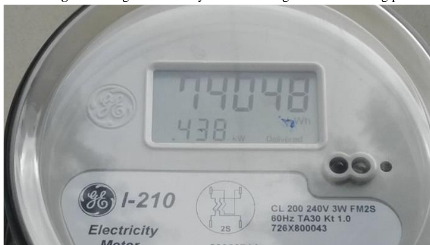
Figure 6. Digital electricity meter showing real-time running power.
