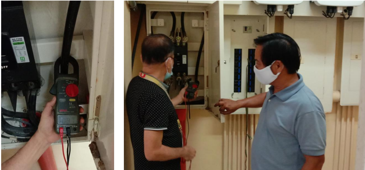
Figure 5. Actual running power (current x voltage) measurements by electrical Engr. Sabas Lazaro and Dr. Januel Floresca, Study Leader.
